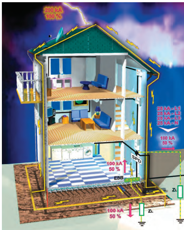
Figure 60: Current sharing in the case of exposed structure and installed external lightning protection system
