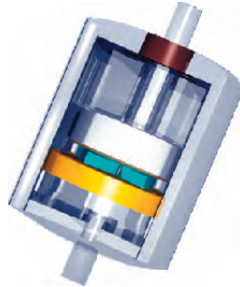
Figure 47: Example of self-extinguishing spark gap
